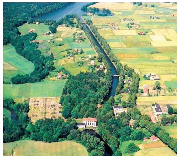
Fig. 2. View to Lake Żurskie with derivation channel and hydropower plant
