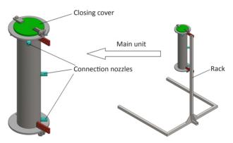
Figure 1 Diagram of the stand for testing the sterilization process of food raw materials
