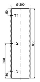
Figure 3 Layout of the temperature sensors: T1, T2, T3
