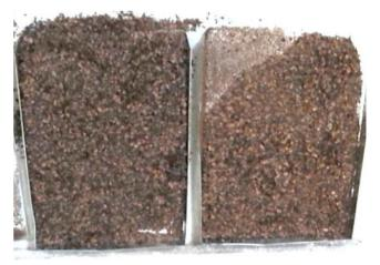
Figure 4 Heat treated cocoa shell (heat treatment time: 2 min). Left side: 300°C, right side: 200°C
