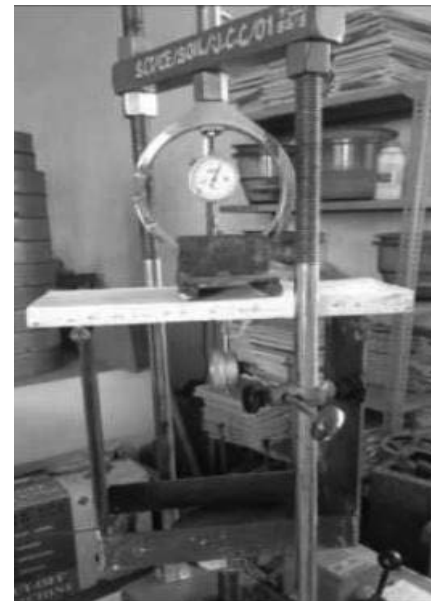
Figure 5. Testing of ferrocement laminates.
