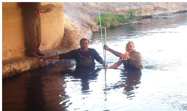
Photo 4. Flow velocity measurements at the centre of the canal (phot. M. Sayah Lembarek)
