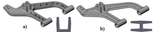
Fig. 3. The proposed two designs of the rocker arm cross-section: a) U-shaped profile, b) I-shaped profile
