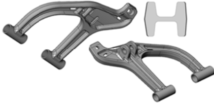
Fig. 5. Model configuration of the lower rocker arm with an I-shaped cross-section.
