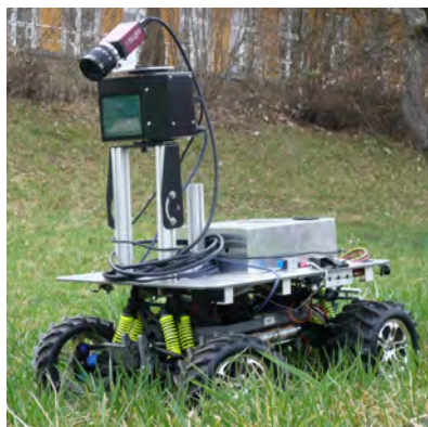
Figure 4. Robot with mounted 3D laser ranging sensor
