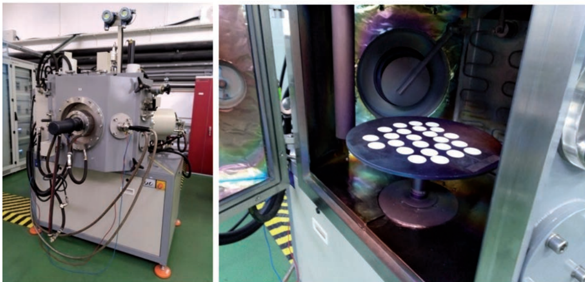
Fig. 2. The chamber used for plasma treatment of polyamide membranes
