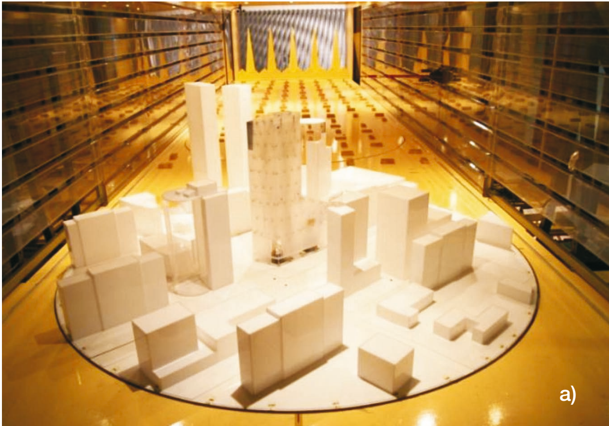
Fig. 5a–b. Building model and the surrounding environment in the measurement space of the wind tunnel. Visualization of the distribution of the average wind pressure coefficient on the external surface; source: A. Flaga 2015, Laboratory of Wind Engineering, Cracow Univ. of Tech. 2013
