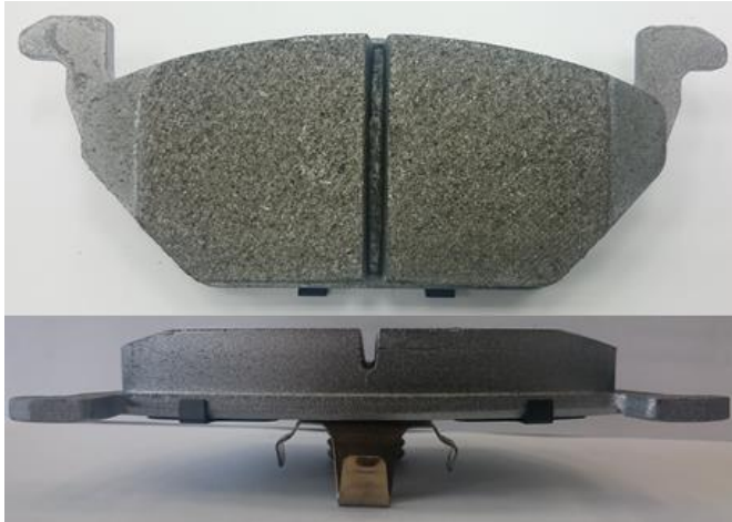
Picture. 7 & 8. The chamfered and slotted brake pad.
