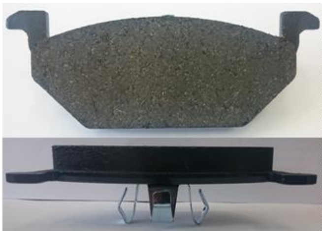
Picture. 1 & 2. The grinded brake pad.
