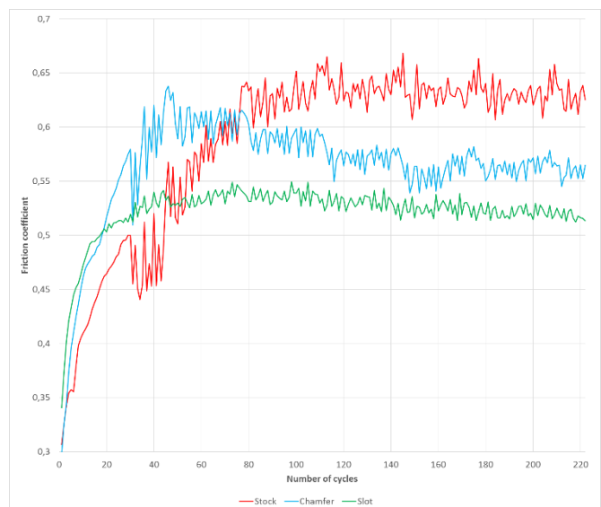
Graph. 1. Burnishing phase test results.
