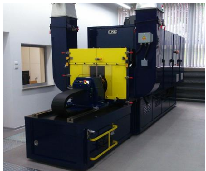
Picture. 9. The LINK M3000 Inertia Brake Dynamometer in BOSMAL Automotive Research and Development Institute Ltd.
