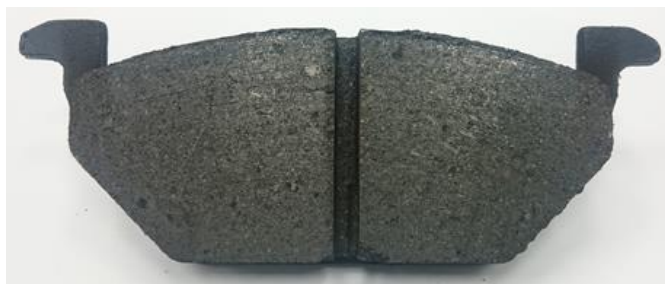
Picture. 12. The Slotted brake pad after the test
