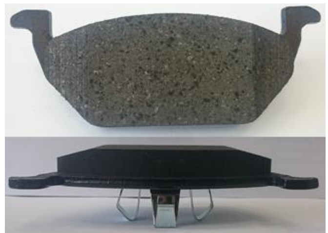
Picture. 3 & 4. The chamfered brake pad.
