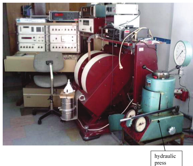
Fig. 5. Photo of the hydraulic press connected to EPR spectrometer from our laboratory
