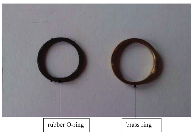
Fig. 8. Photo of high pressure seals used in our laboratory: on the left – a rubber O – ring, on the right – a brass seal
