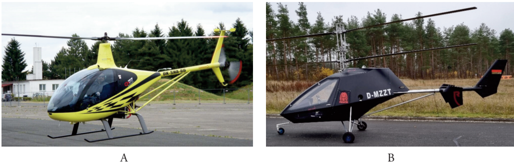
Figure 1. The small weighted helicopter. (A) Single-rotor helicopter Ranabot CH-77 (Italy), MTOM-500 kg, (B) coaxial helicopter Rotorschmiede VA-250 (Germany), MTOM-500 kg.
