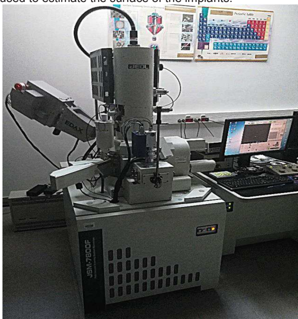
FIG. 1. Scanning electron microscope JSM-7800F.
