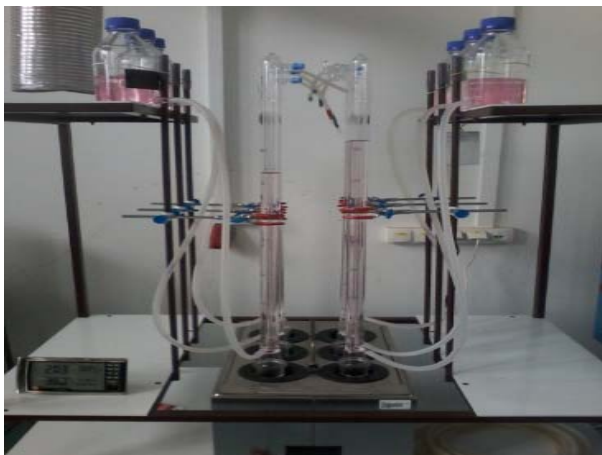
Fig. 2. DIN 38414/8 eudiometers used for small-scale (400 mL) experiments including water bath, Testo 622 instrument for temperature and atmospheric pressure measurements table specially designed for this purpose.
