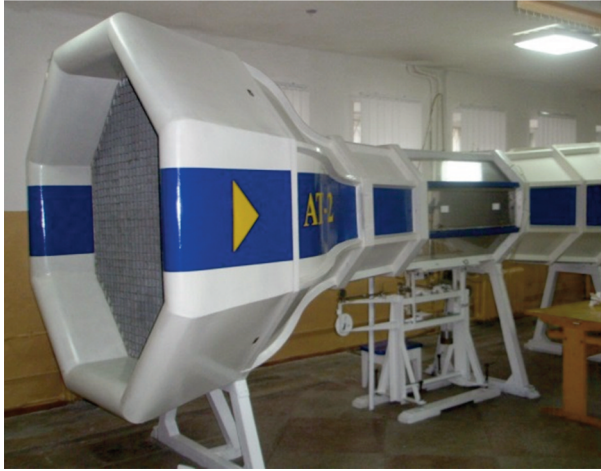
Fig. 1. Wind tunnel AT-1 Research Institute of Aviation [Lemko; 2010]
