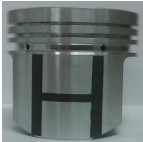
Fig. 1. Piston with an H-shape coating layer
