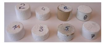
Fig. 5. Ceramic samples prepared for measurements in the impedance tube with diameter 29 mm; the samples 5 and 6 are made up with plaster, whereas the samples 7 and 8 are wrapped up in a thin tape in order to fit well in the tube.
