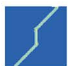
Fig. 14. Pre-crack damage and crack propagation for different pre-crack angles
