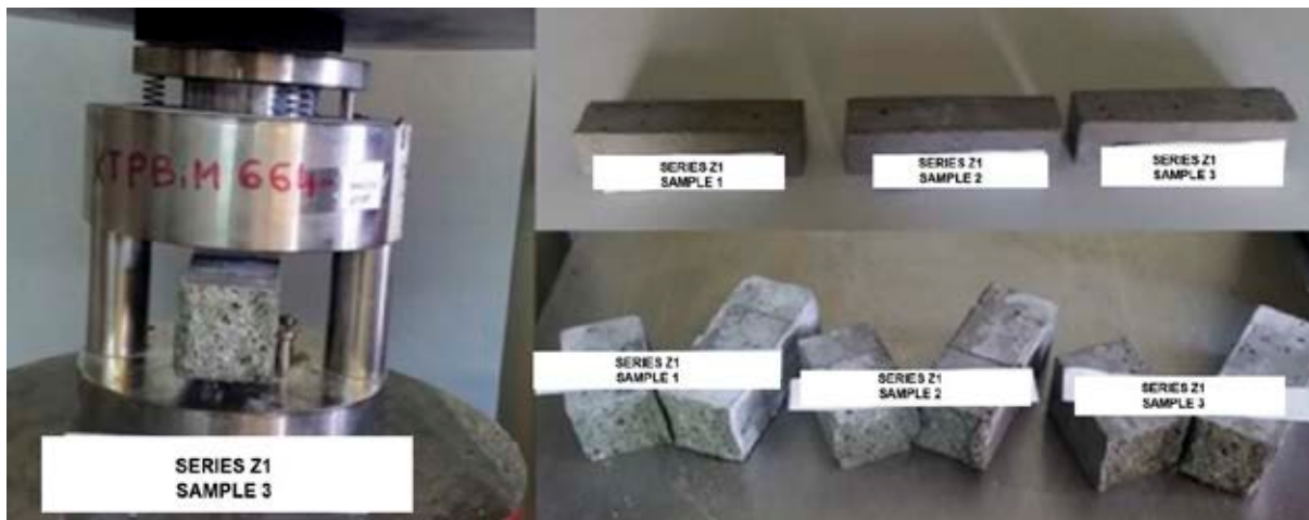
Figure 3. Strength tests of cement mortar beams
