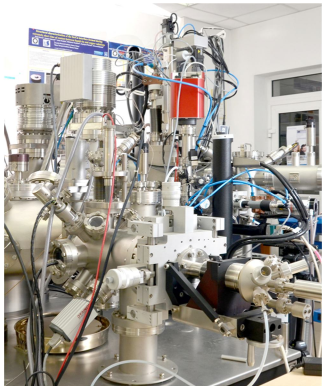
Fig. 1. View of the apparatus for placing drops of metal on the moulding sand substrate
