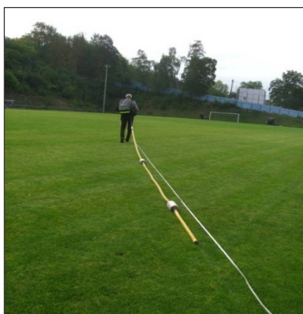
Fig. 5. Measurements with the GPR method with a 50MHz non-screen antenna, diagonal profiling
