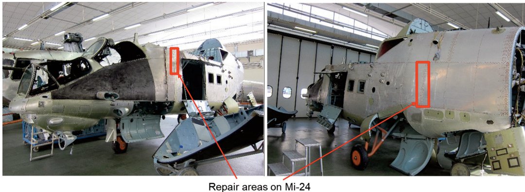
Fig. 3. Pictures of repair areas on Mi-24.
