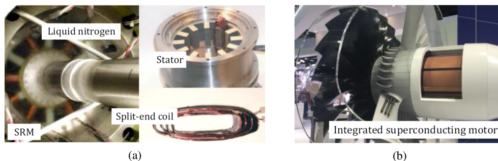
Fig. 6. Examples of cryogenically-cooled machines: (a) SRM demonstrator with conventional Cu winding – NASA [33]; (b) integrated superconducting motor for aerospace propulsion – ASuMED project [35]
