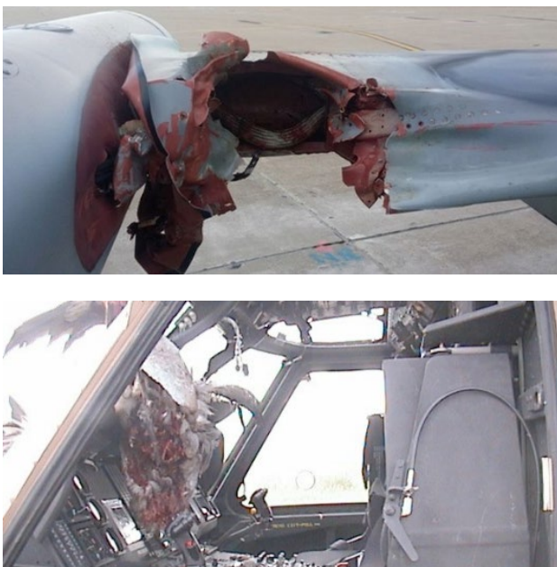
Fig. 3. Examples of the consequences of a collision between an aircraft and a bird. Above, an example of a collision between a Czech L-159 fighter and a vulture 1 . Below, an example of a Sikorsky UH-60 Black Hawk helicopter colliding with a common crane 2
