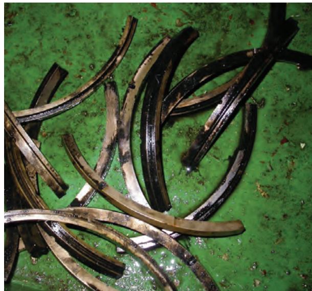
Fig. 6. Broken piston rings of main engine
