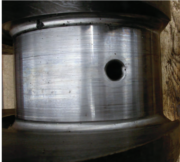
Fig. 7. Unacceptably worn of crank pin of the auxiliary engines delivered residual fuel and operated under tropical conditions
