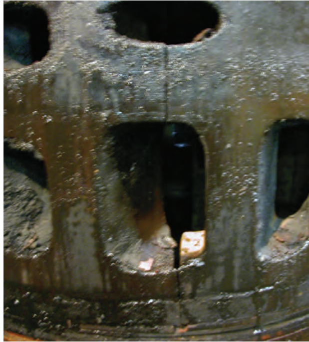
Fig. 5. View of cracked cylinder liner
