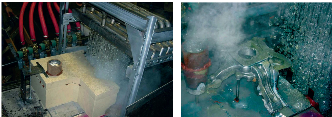
Fig. 1. Ablation casting presented by Alotech, Co. [7]
