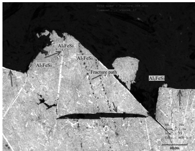
Fig. 5. Cross section of fractured surfaces of AA 4032 alloy showing fracture mechanism of Al_5FeSi intermetallic phase
