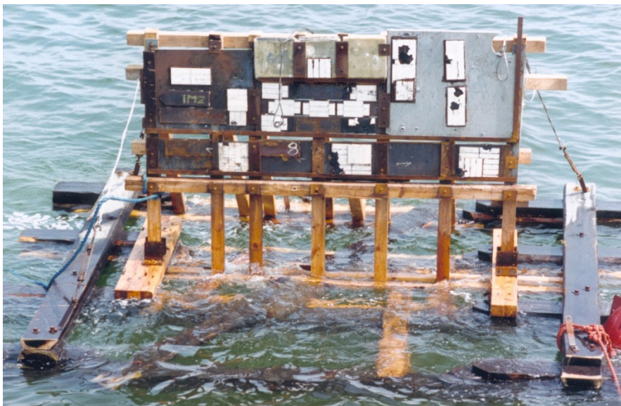
Fig. 6. Floating shield after shelling on the training ground sea [from the author's archive]
