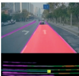
Fig. 10. Determining line segments using a video camera and IMU [adapted from [50]]
