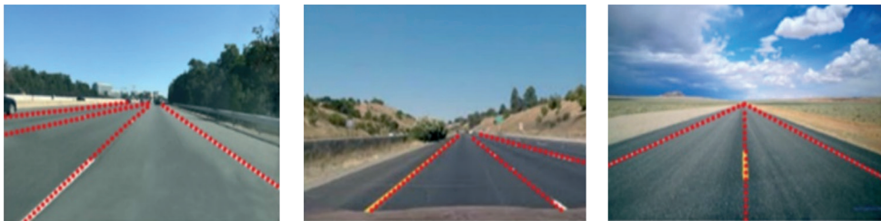
Fig. 21. The way to determine the lanes by establishing the points associated with the traffic lanes in different environmental situations, by the method proposed in [66]
