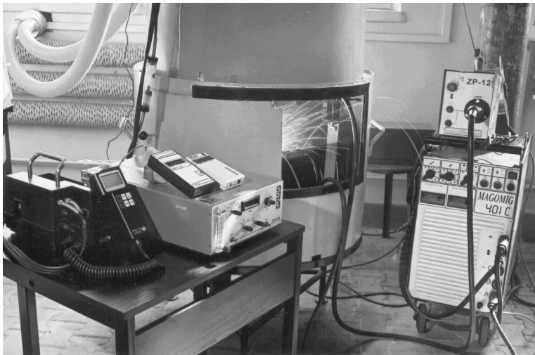
Figure 2. Test station for investigating dust and gas emission during tubular cored wire welding.
