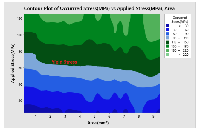
Fig. 5. Contour Plot of generated Stress vs Applied Stress per area of the pore
