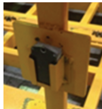
Fig. 6. The FIX case for positioning of IRFID chip
