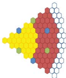
Fig. 2. ELFR core configuration with INN (yellow) and OUT (red) FA positions surrounded by dummy elements (white). Blue and green hexagons represent control and shutdown assemblies, respectively.
