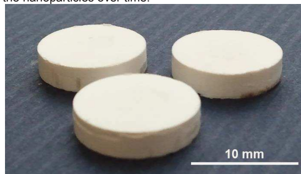
FIG. 1. Test molds of pure BCP before modification with nanometals.
