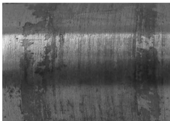
Fig. 9. Macroscopic image of the uncoated shaft top layer
