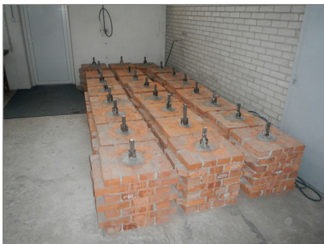
Photo 10. Test specimens modelling brick foundations
