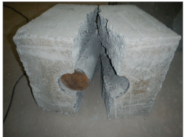
Photo 9. Pile after concrete specimen failure
