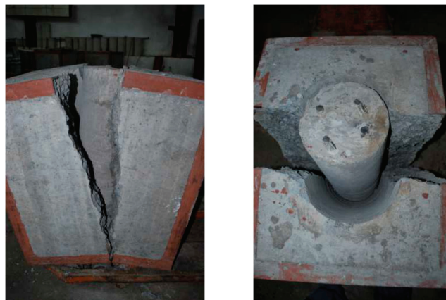
Photo 2. Form of specimens failure
