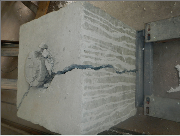
Photo 7. Form of concrete specimens failure
