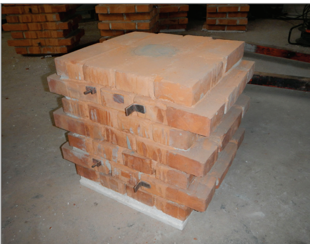
Photo 4. Specimen modelling foundation made from brick
