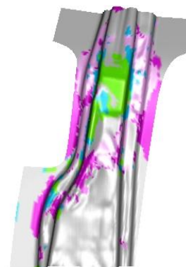
Fig. 4. B-pillar drawn from the simple blank with highlighted strain areas
