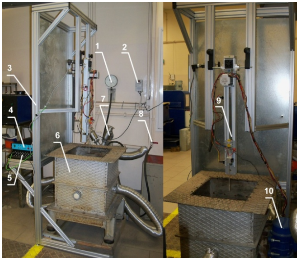
Fig. 3. The testing bench for forming and casting (real view) 1 – vacuum gauge, 2 – inverter, 3 – stator, 4 - SSK-1 controller , 5 - MP16B type convertor, 6 – mould flask with perforated bottom, 7 – vacuum device valve, 8 – compressed air device valve, 9 – MLA-SK linear module, 10 – mechanical electric vibrator
