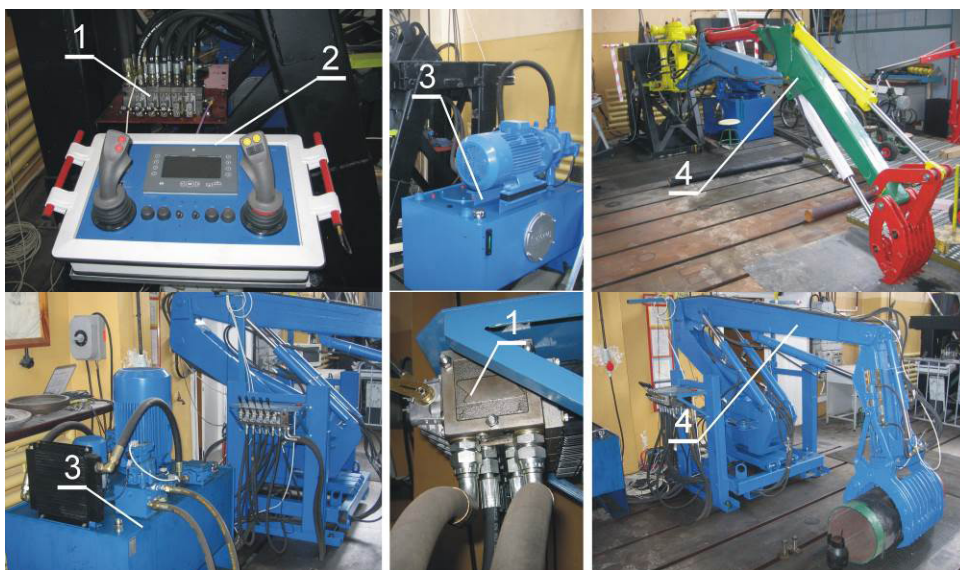
Fig. 1. Test stations for testing control systems using the CAN bus: 1 – hydraulic valve with electronic CAN-bus modules, 2 – remote control desktop, 3 – hydraulic power unit, 4 – work tools
