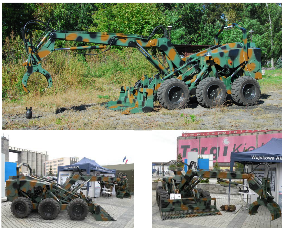
Fig. 10. Engineering support robot EOD/IED "Marek"
