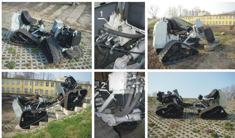
Fig. 8. Unmanned land platform with control based on a CAN: 1 – hydraulic valve, 2 – electronic CAN-bus modules
