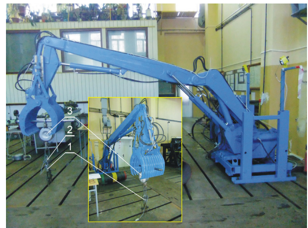
Fig. 5. Test station for measurement of load force of engineering support robot manipulator (description in the content of the text above)
