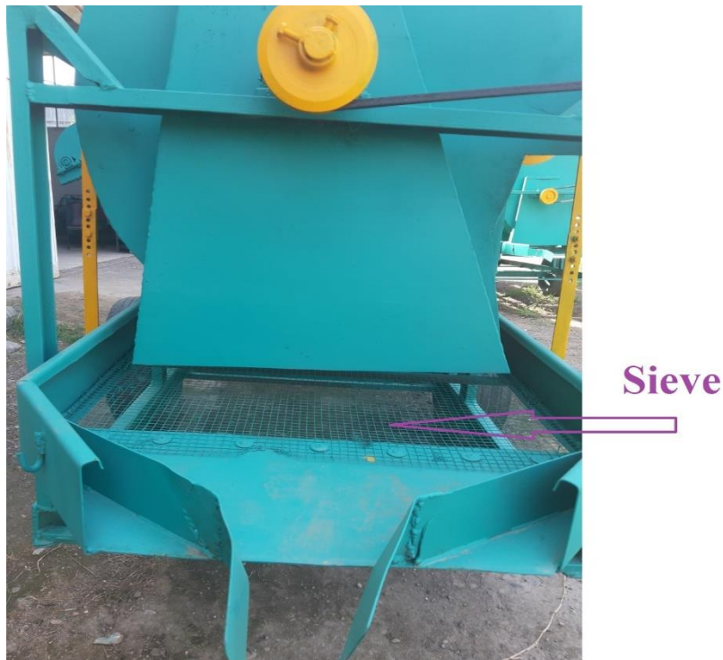
Figure 4. Sieve in the separation section
