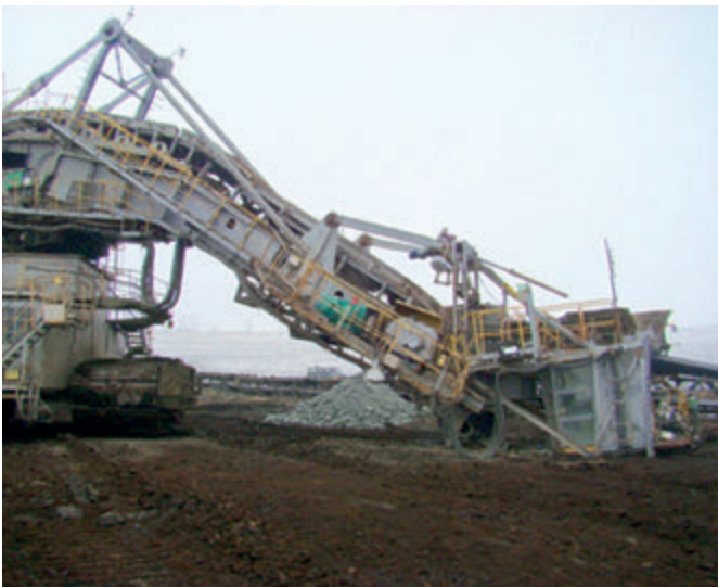
Fig. 2. Disaster of BWE SRs 1200 at lignite open pit mine Konin [6] Rys. 2. Katastrofa koparki kołowej SRs 1200 w KWB Konin [6]
