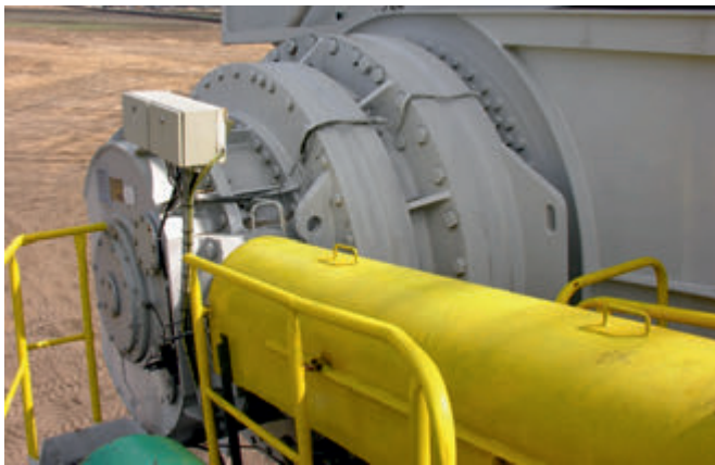
Fig. 10. Planetary gear of modernized drive of bucket wheel in BWE KWK 1500s at lignite open pit mine Konin
