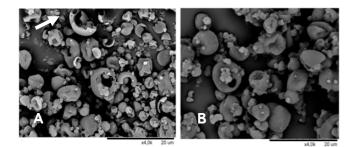
Fig. 4. SEM pictures of powders obtained by spray drying of emulsions with 80:20 water to oil ratio and A) 10% and B) 20% lactose concentration in the aqueous phase. Scale bar -  $20 \mu m$ .
