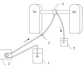
Fig. 1. The experimental set-up for determination of droplet size in O/W emulsions. 1- vessel with a pure water, 2- peristaltic pump, 3 - sample injection point, 4 -wet measurement cell, 5 - waste collection beaker, 6a - Spraytec laser detision unit. b - Spraytec laser detection unit
