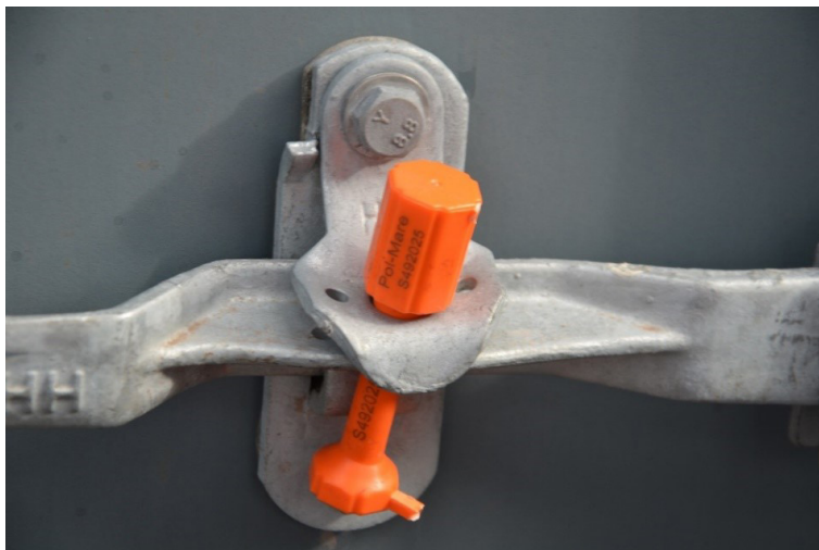
Figure 5. Securing the container closure with a bottle seal [7]
