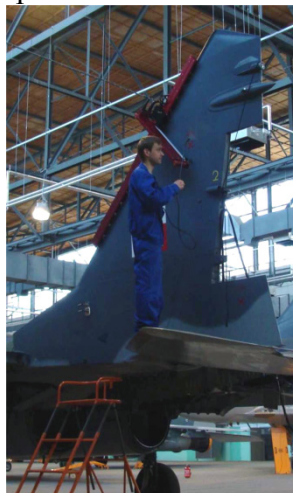
Pic. 1. Composite vertical stabilizer inspection.
