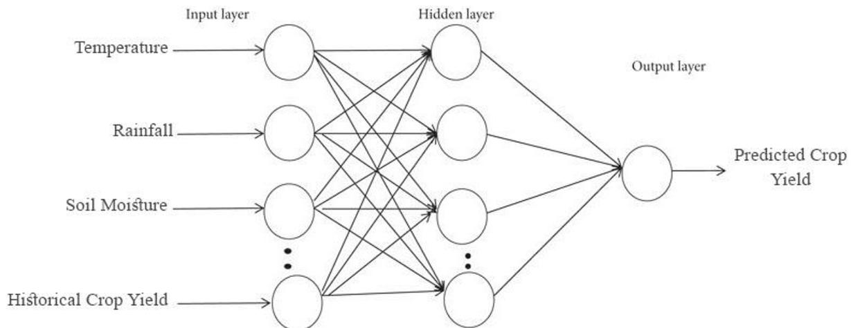
Figure 3. Architecture of the FFANN with the single hidden layer
