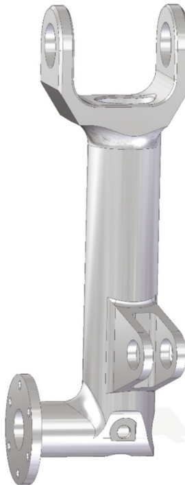
Figure 12. Design of lever from steel material.
