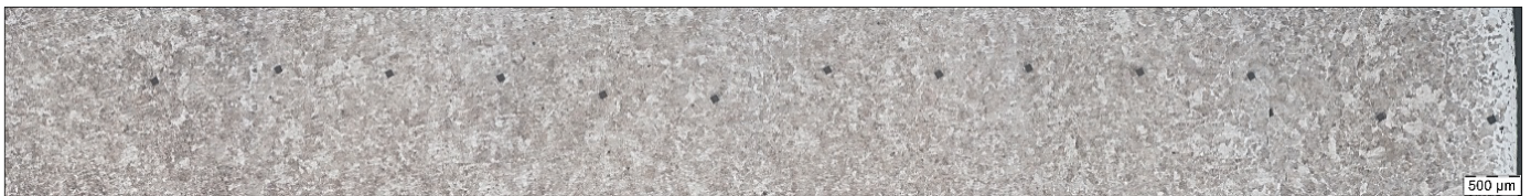
Fig. 19. The microstructure of forgings for the annealing temperature of 680°C and isothermal holding time 1.0 h
