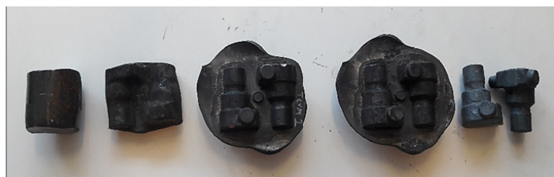
Fig. 5. Appearance of forgings after each forging operation
