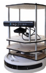
Figure 6. A TURTLEBOT with a laser scanner
