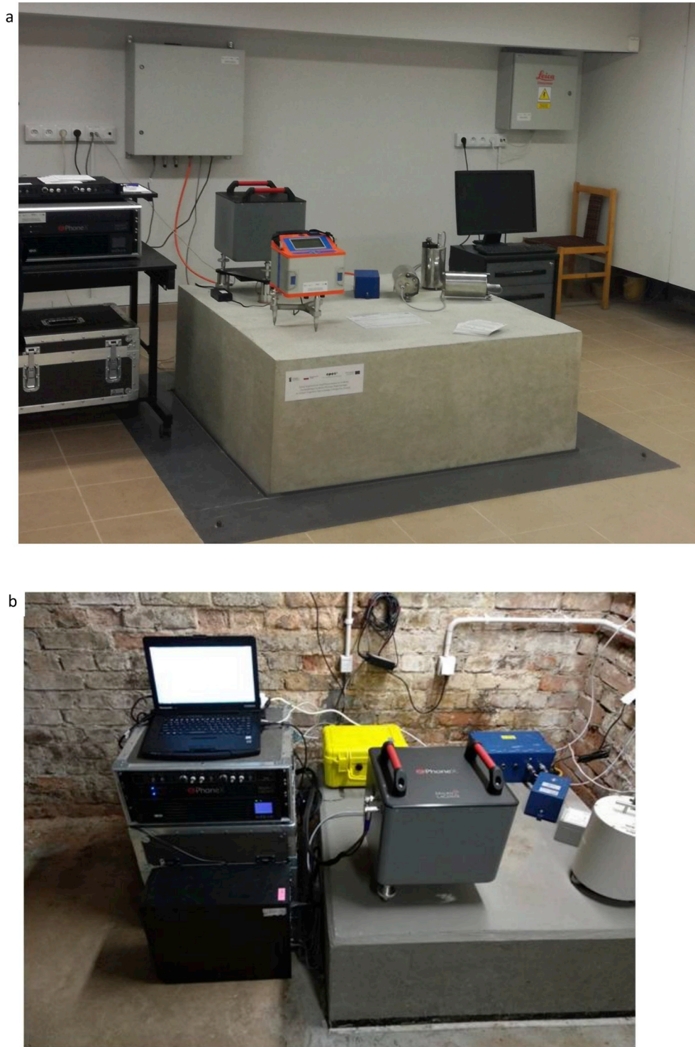
Fig. 8. Photos of geophysical stations at GIG in Katowice (a) – on pedestal are seen gravity meters CG-6, gPhoneX, 5 s GeoSIG seismometer and 1 s Willmore's MKIII seismometer and at "Ignacy" Historical Mine in Rybnik (b) – on pedestal are seen gPhoneX gravimeter, 5 s GeoSIG seismometer and rotational R1 angular velocity sensor.
