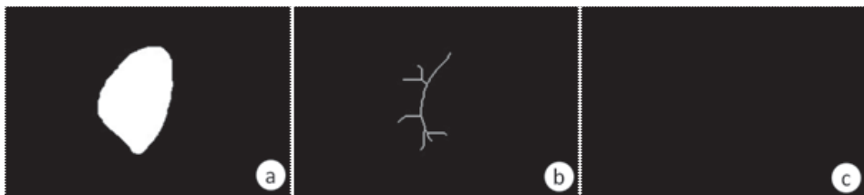
Fig. 3. a) test image (fig. 2 a) after close-hole operation; b) skeleton of the image a; c) skeleton after an “infinite” (in this case — 25) iterations of pruning
