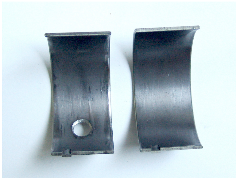
Fig. 2. Surfaces of new half-bushes with sliding layers made of MB58 alloy before testing in the SMOK rig [9]
